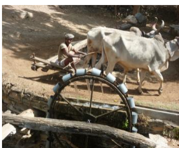
Traditional groundwater lifting in India
